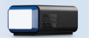
Sensitive area (width x height)  $[mm^2]$  77.2 x 38.6 (Brandeis detector was 86 x 49 mm<sup>2</sup>) Pixel size  $[\mu m^2]$  75 x 75 Number of pixels (horiz. x vert.) 1030 x 514 = 529,420 Maximum frame rate [Hz](30 s burst) 9000 Maximum frame rate [Hz] (continuous) 3000 Readout time  $[\mu s]$  continuous readout, 3  $\mu s$  dead time Point-spread function 1 pixel Maximum count rate [phts/s/mm<sup>2</sup>] 5 \* 10<sup>8</sup>
